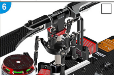
Check linkage rod and ball of main rotor head and tail rotor head.
